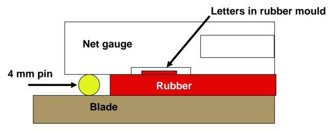
b) If the ruler touches the pin and the far side of the rubber (as shown below), it is less than 4.0 mm thick and the result should be recorded.
