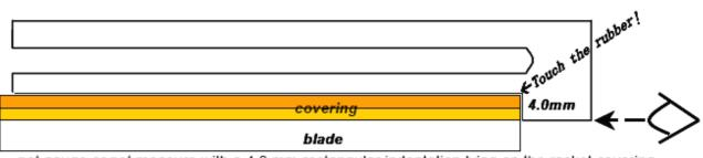
net gauge or net measure with a 4.0 mm rectangular indentation lying on the racket covering
