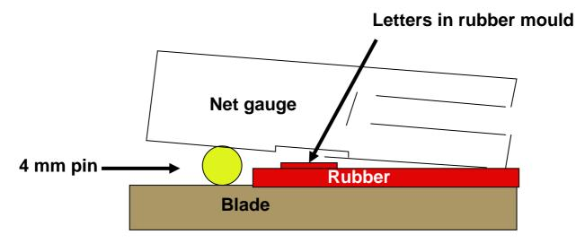
c) If the ruler touches the rubber, but not the pin, the rubber is too thick (as shown below). The gap between the ruler and the pin can be measured using a thickness gauge. The
