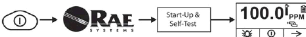
6. When the display shows "Ready ... Start sampling?" press the Y/+ key to start the measurement.
