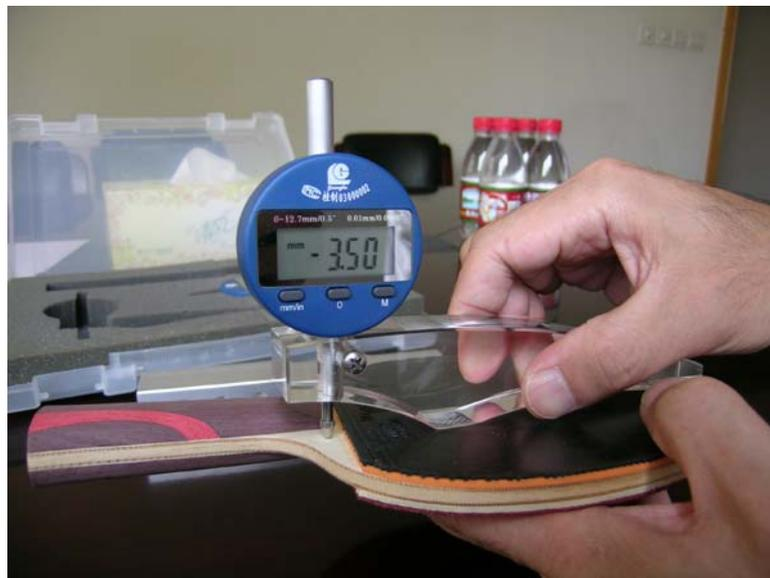
The diameter of the pin touching the blade shall be between 04.5 and 05.0 mm.
